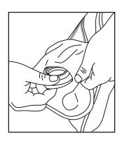
Remove the original T-Piece base (RB03/03) and protector (RB03/04) from the bladder
