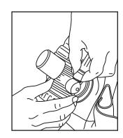
12. Fit the regulator hose to the diluent 1st stage or manifold and the ADV swivel
