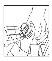
8. Insert the BS130N70 o-ring (provided) into the T-piece base
