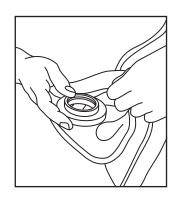
6. Carefully insert the new T-Piece base (RB03/03) and protector (RB03/04) into the bladder and re-fit to the outer bag
