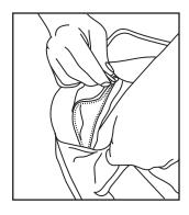
Unzip the outer bag on the back of the counterlung to gain access to the bladder
