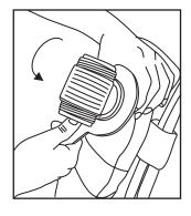
2. Remove the T-Piece with the C Spanner provided
