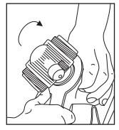
Tighten the locking ring with the C spanner and re-attach the blue ring and buzzer
