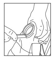
Push outer bag to the base of the thread using the C spanner handle whilst pulling material taught around fitting
