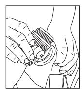
Place the T-piece onto the base and screw down locking ring
