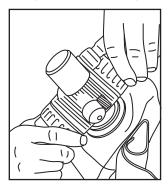
Re-attach the breathing loop hoses to the T-piece with the swivel connector on the outside
